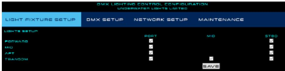
You can have up to nine differently addressed fixtures. If required, it is permissible to leave gaps in the scheme so that the mimic diagram matches the physical layout on the vessel.
